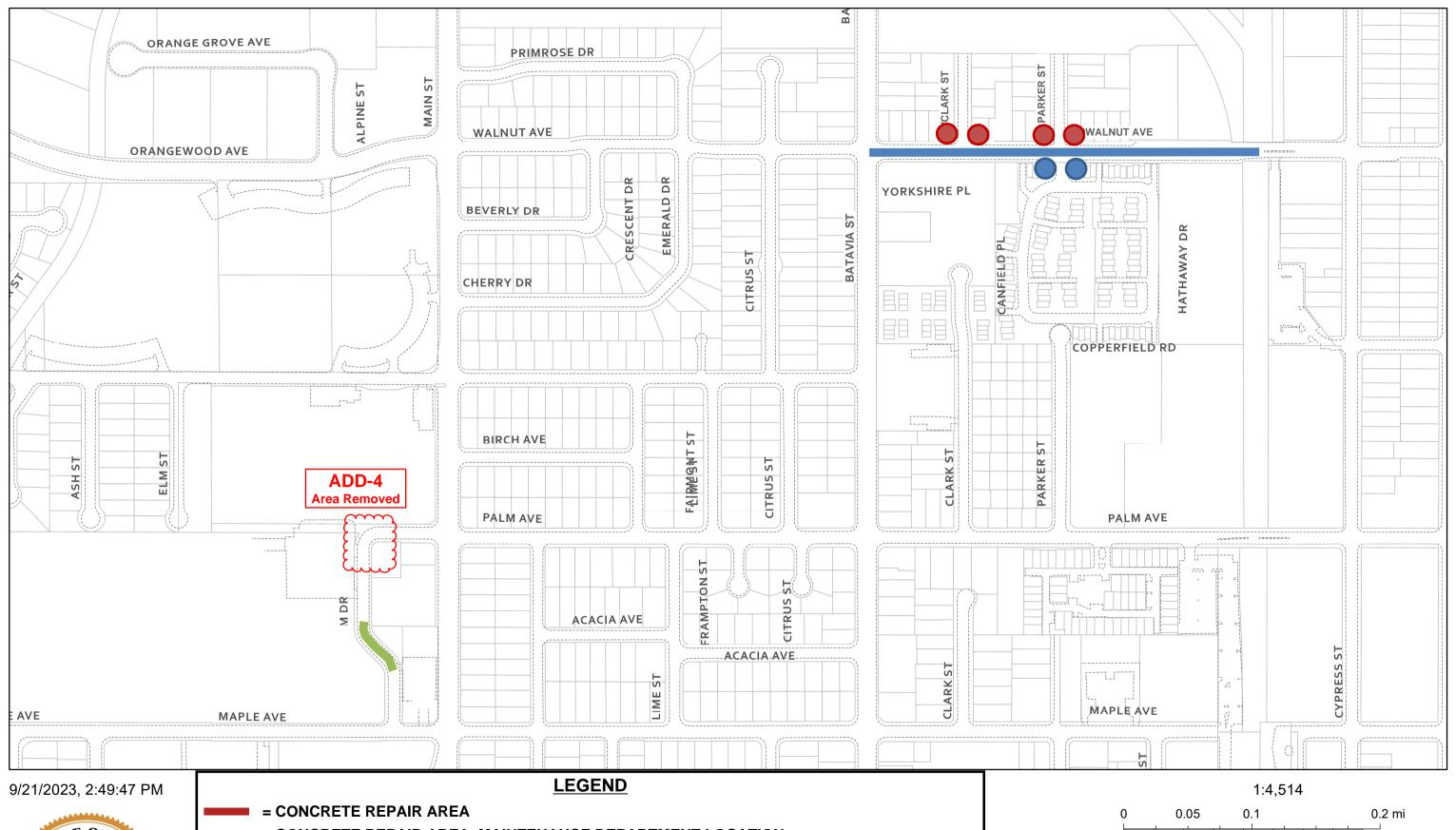
OF ORATES CE = CONCRETE REPAIR AREA, MAINTENANCE DEPARTMENT LOCATION = SPECIAL REPAIR AREA, CURB REPLACEMENT WITH CURB & GUTTER, SEE PROJECT PLANS = PLAZA BRICK REPLACEMENT AREA, SEE PROJECT PLANS OPARIL 6, 1888 CALIFOR = REPLACE CURB RAMP, TYPE PER ADA RAMP TABLE = REPLACE RAMP TRUNCATED DOMES ONLY = REPLACE CURB RAMP, SEE RAMP LAYOUT DETAILS = REPLACE CURB RAMP AFTER STREETLIGHT RELOCATION, SEE RAMP LAYOUT DETAIL
