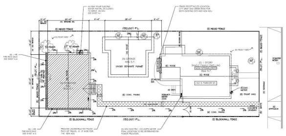
Site plan showing proposed location of new detached ADU (not to scale; Allstar Design and Engineering Group)
