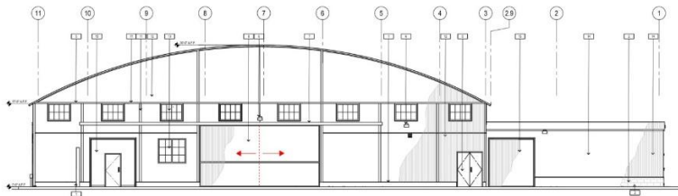
Figure # 7: east secondary façade existing conditions; AO Drawing shows original location of bi-parting sliding corrugated metal door panels noted with red directional arrows.
