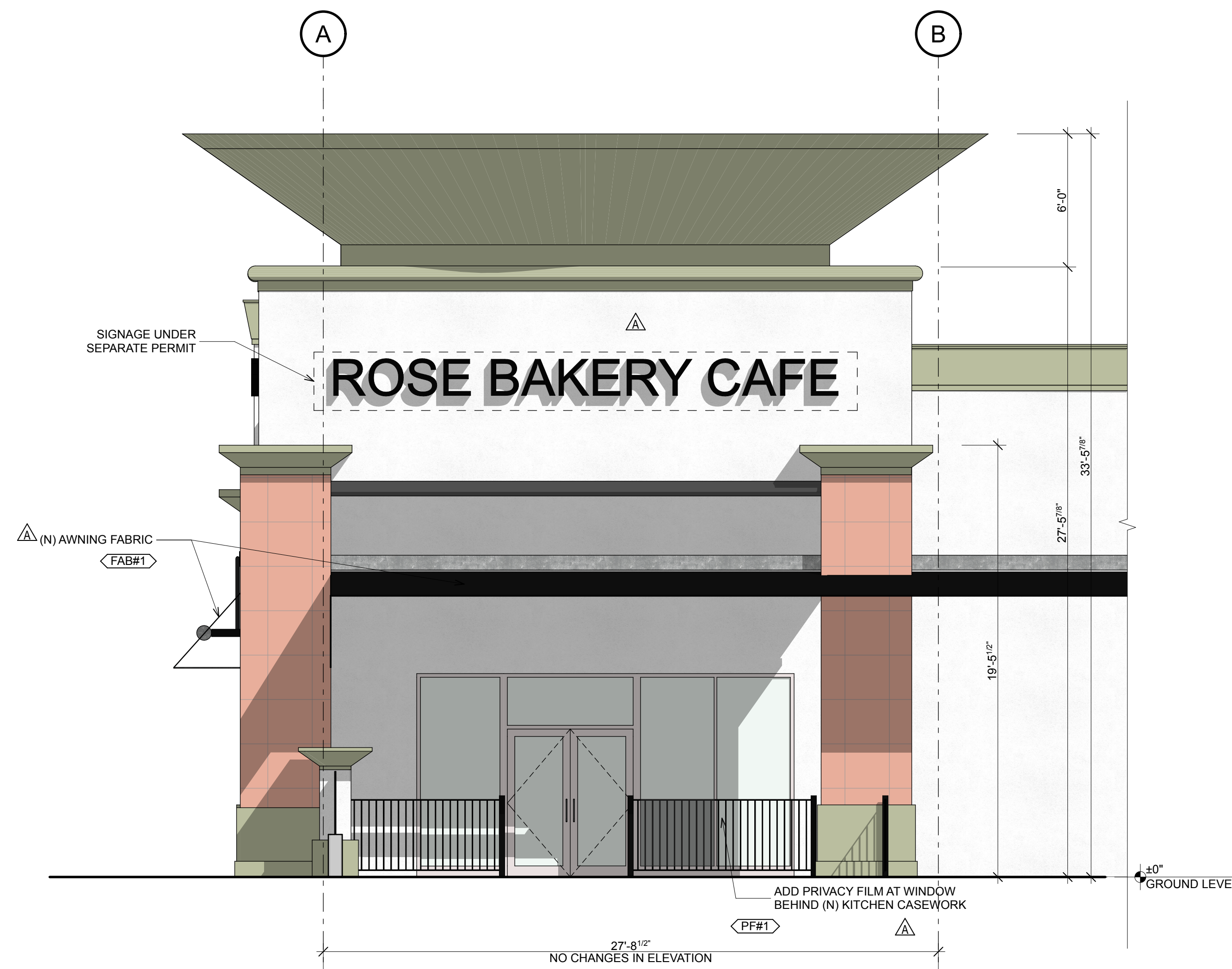
A EXTERIOR ELEVATION (EAST)
