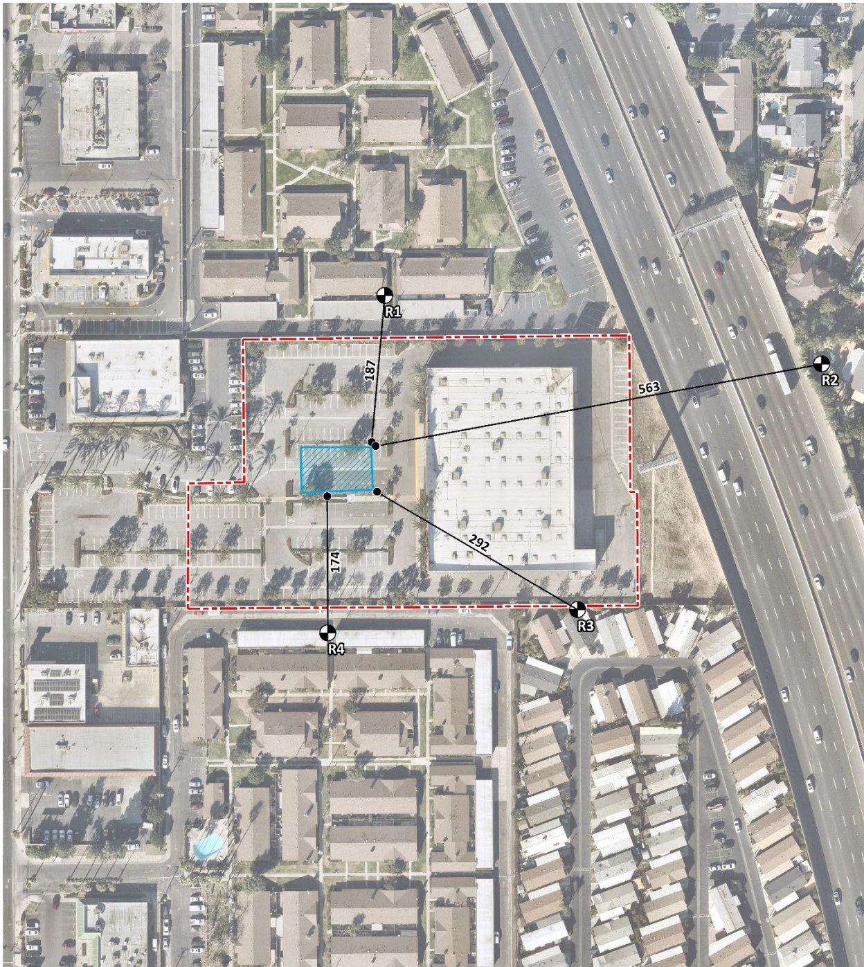
Figure N-3: Concrete Crushing Activities and Sensitive Receiver Locations
