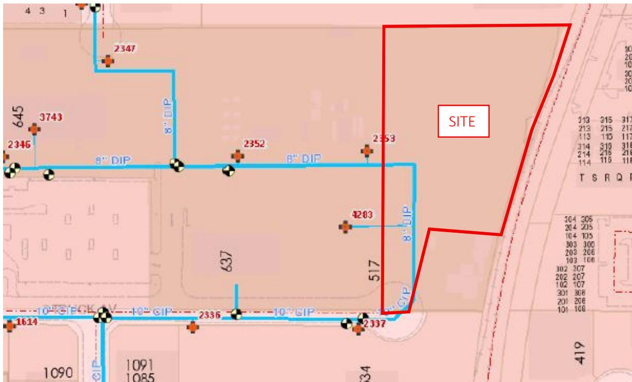
A flow test was performed by SoCal Flow Testing on 3/18/20 on the nearest fire hydrant (2nd hydrant east of N Parker St on south side of W Struck Ave). The static pressure in the 10" main in Struck Avenue was 82 PSI, the 2-1/2 inch nozzle flow rate was 1,256 GPM with a residual pressure of 55 PSI. The calculated flow at 20 PSI residual is 4,432 GPM.
