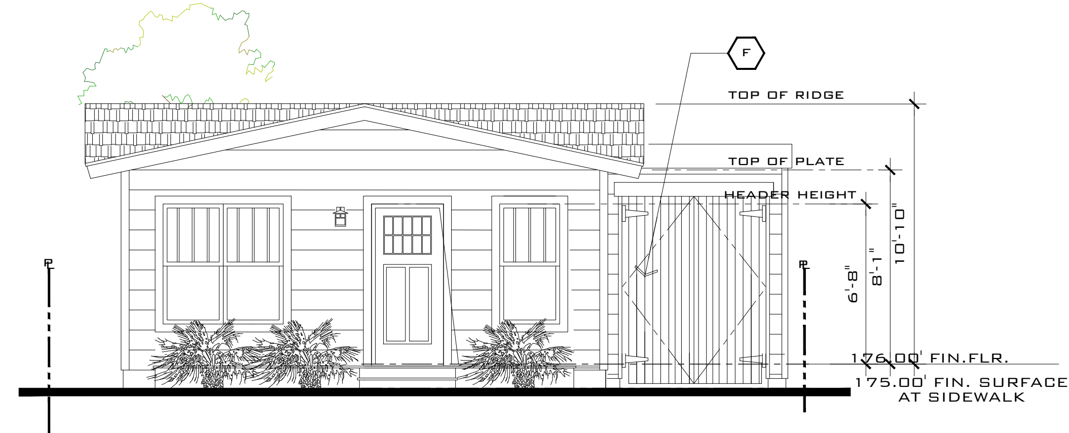
PROPOSED EAST FRONT ELEVATION SCALE: 1/4" = 1'-0" SEE SOUTH ELEVATION FOR FINISH MATERIALS - TYPICAL
