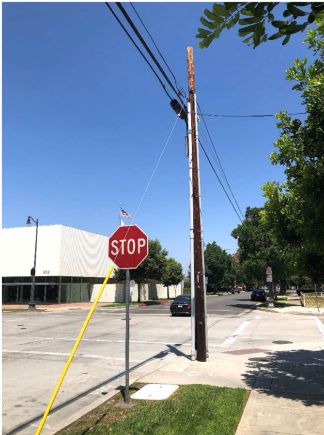
This utility pole may create some signal pole placement and line of sight issues. We will verify signal pole location and clearance with the City
