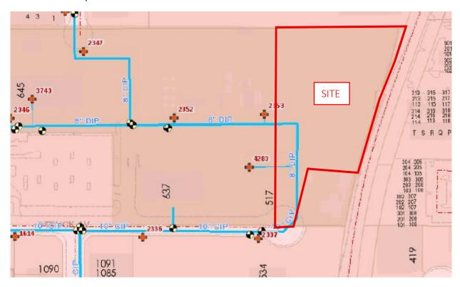
A flow test was performed by SoCal Flow Testing on 3/18/20 on the nearest fire hydrant (2nd hydrant east of N Parker St on south side of W Struck Ave). The static pressure in the 10" main in Struck Avenue was 82 PSI, the 2-1/2 inch nozzle flow rate was 1,256 GPM with a residual pressure of 55 PSI. The calculated flow at 20 PSI residual is 4,432 GPM.
