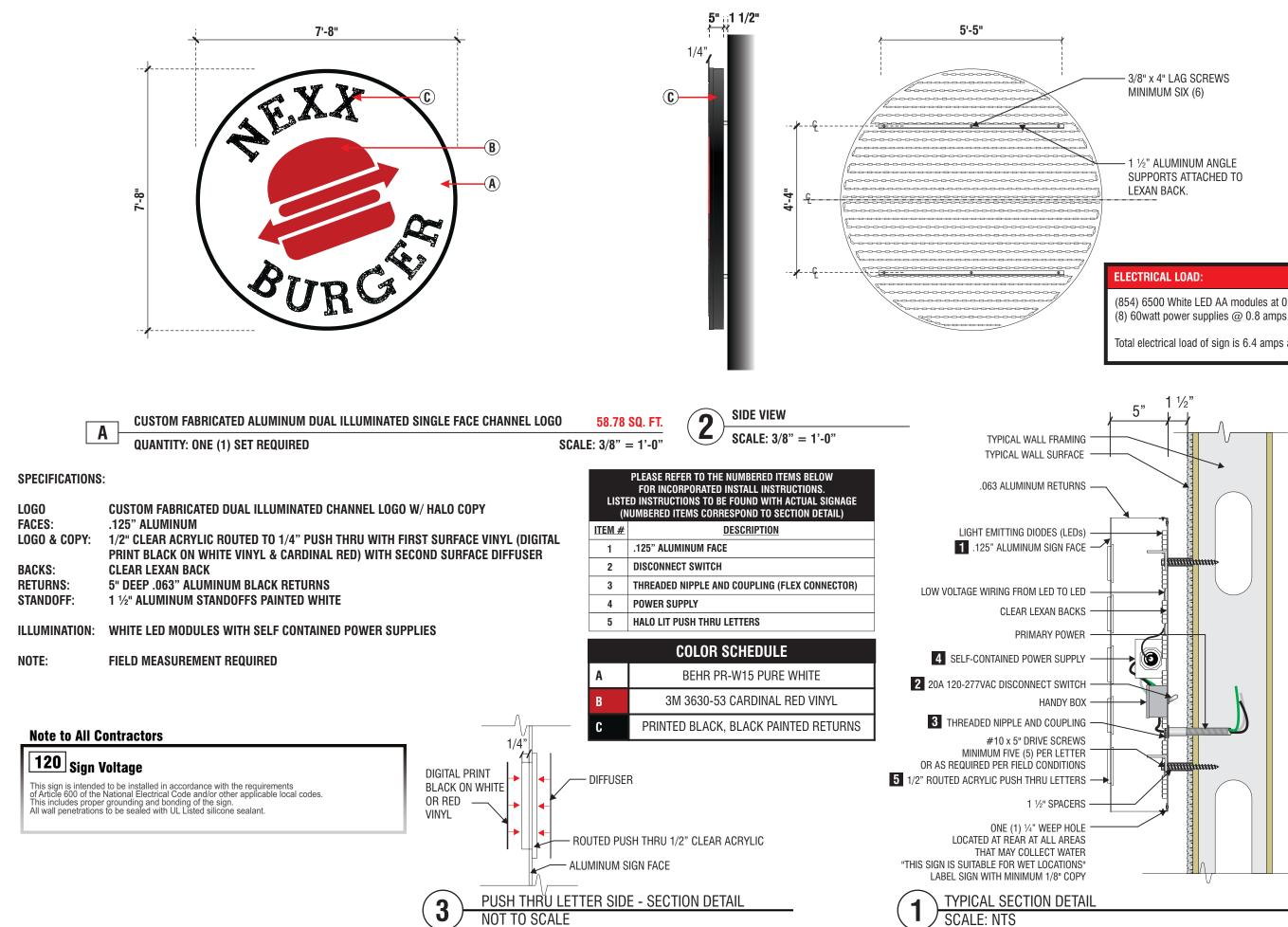
(854) 6500 White LED AA modules at 0.5 watts each (8) 60watt power supplies @ 0.8 amps each.
