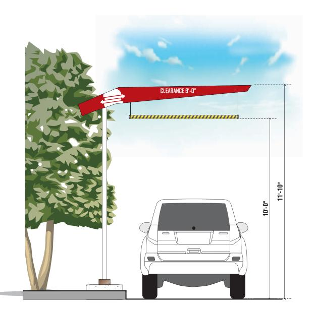
SIDE VIEW - DRIVE THRU CLEARANCE BAR
