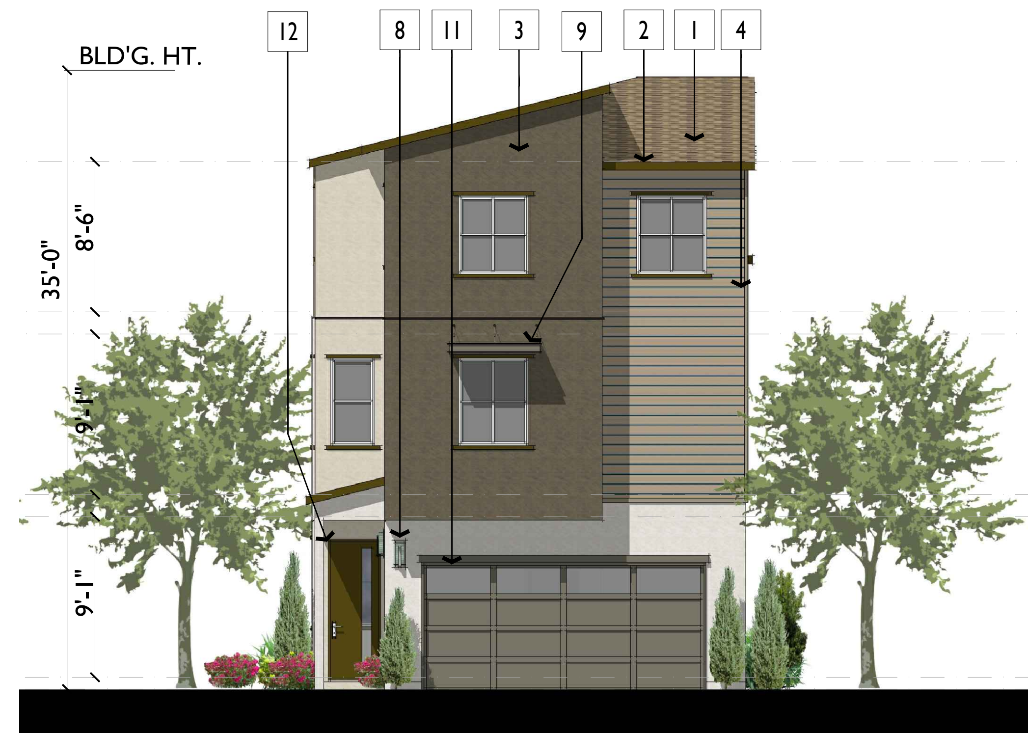
FRONT - DRIVE AISLE ELEVATION
